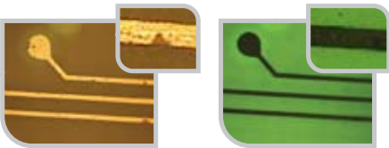
Oxidation false calls as imaged with UV illumination
